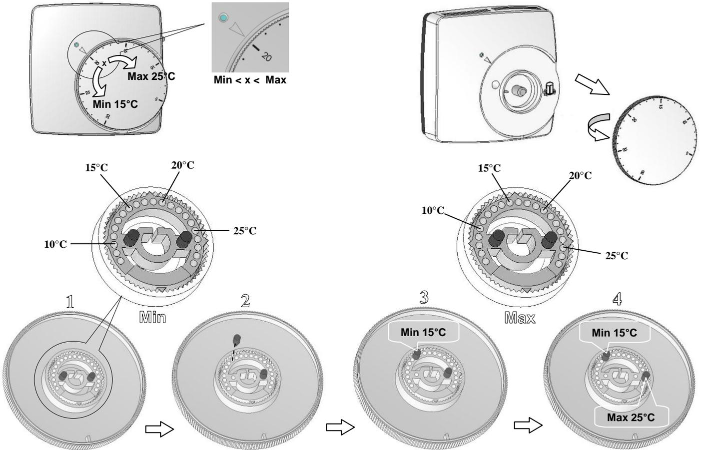
**F** Calibration    **GB** Calibration    **D** Kalibrierung    **I** Calibrazione    **E** Calibración
