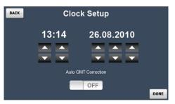
Here you can set the current time and date and select whether the Touchpad should observe GMT Correction. GMT correction will automatically change the clock on the Touchpad and Thermostats in March and October as the clocks change for Winter/Summer time.
